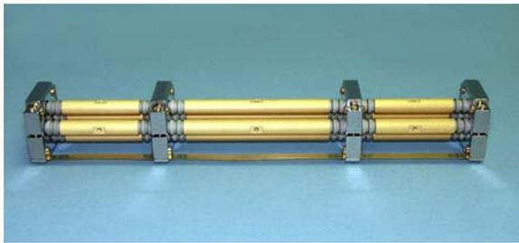
**Fig. 2.** The electrostatic triplet lens. The lengths of the sections are related to the electric field strengths required for focusing so that all voltages are similar in magnitude. Two of these lenses one meter apart make up the compound lens.
