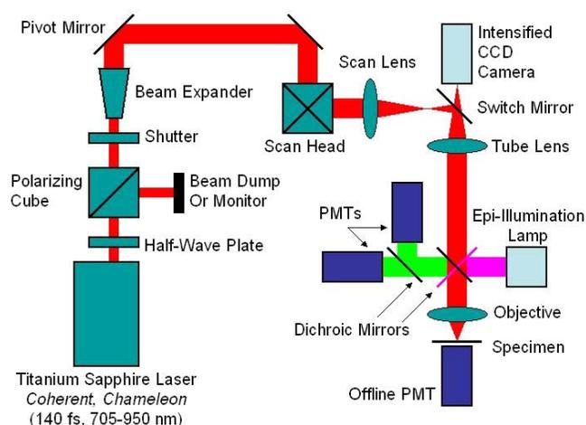
**Fig. 4.** Diagram of the multiphoton microscope optics path.
