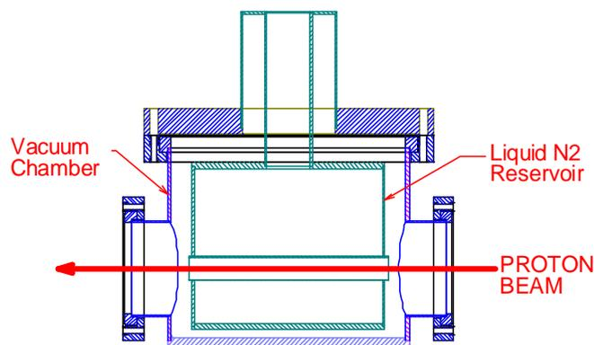
**Fig. 1.** Design of the liquid nitrogen trap for the oxygen/nitrogen resonance explosives detector.
