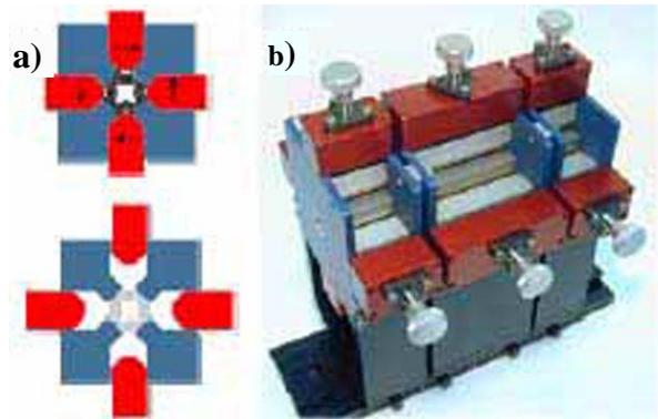
**Fig. 3.** Permanent magnet quadrupole triplet: a) Adjustment of the field by moving the magnets in and out. b) Triplet.
